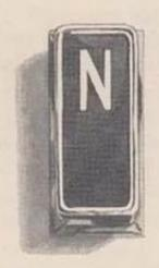
Neutral—push to disengage the gears after parking
